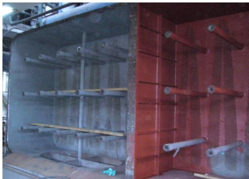
**Fig. 2.** Cooling water inlet chambers.
