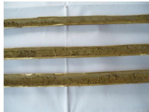
**Fig. 4.** Build-up of material inside condenser pipes.
